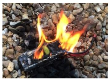
The battery in question was a 2 cell (7.4v) 4000mah LiPo. One of a pair that I use in my Twinstar.
