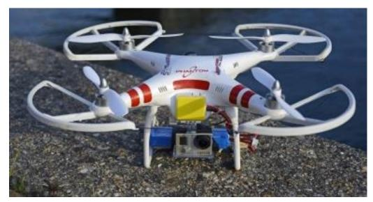
Brian flies an original Phantom 1 (there's a Phantom II out now). It uses 3s 2200-3500mah LIPO batteries that give 5-10 minutes duration. The basic Phantom is a GPS stabilised quadcopter, which allows the machine to be flown in three modes:
