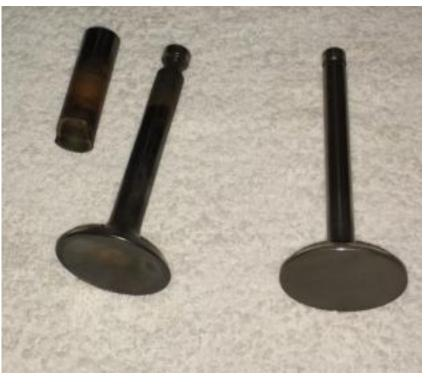
job but with no valve seat, the valve was being slammed into opening around where the seat had been. This caused the valve to "dish" over and was close to being snapped off its stem.
