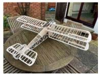
It's not been a very straightforward build, initially due the numerous errors on the 1980's Radio Modeller plan. Unfortunately the laser cut parts had been taken from the plan and many were just hopelessly wrong! The rear fuselage formers were completely unusable and even the wings are drawn one side longer than the other, with the rib spacing all over the place! The icing on the cake was the 152 wing riblets. All too small! To be fair to the designer, Elwin Sapecote (such
