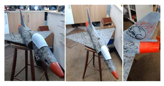
This the other one (below) that I just finished printing, it will have a pusher engine and prop, I have yet to paint it and put everything in it but it already looks pretty good. It's printed with light weight PLA plastic filament at £35 a roll so not cheap but I can just about get 1 plane out of a roll.
