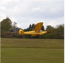
Below see.. Keith's 'scratch' built model, with homemade foam wings, he actually cut them using a li-po battery powered hot-wire. The original 'plan' was reputed to produce a very 'twitchy' model so Keith added a few inches to the fuselage to soften it's flight characteristics, 'success' she flies beautifully.
