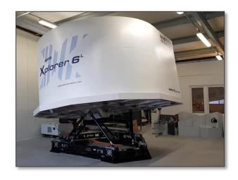
The type specific nature, combined with the accuracy of the hardware and software, allows for specific jet aircraft training to be conducted in the device using in most cases the factory Flight Crew Operating Manual for flight and ground training as well in most cases the actual checklists and Quick Reference Handbooks.
