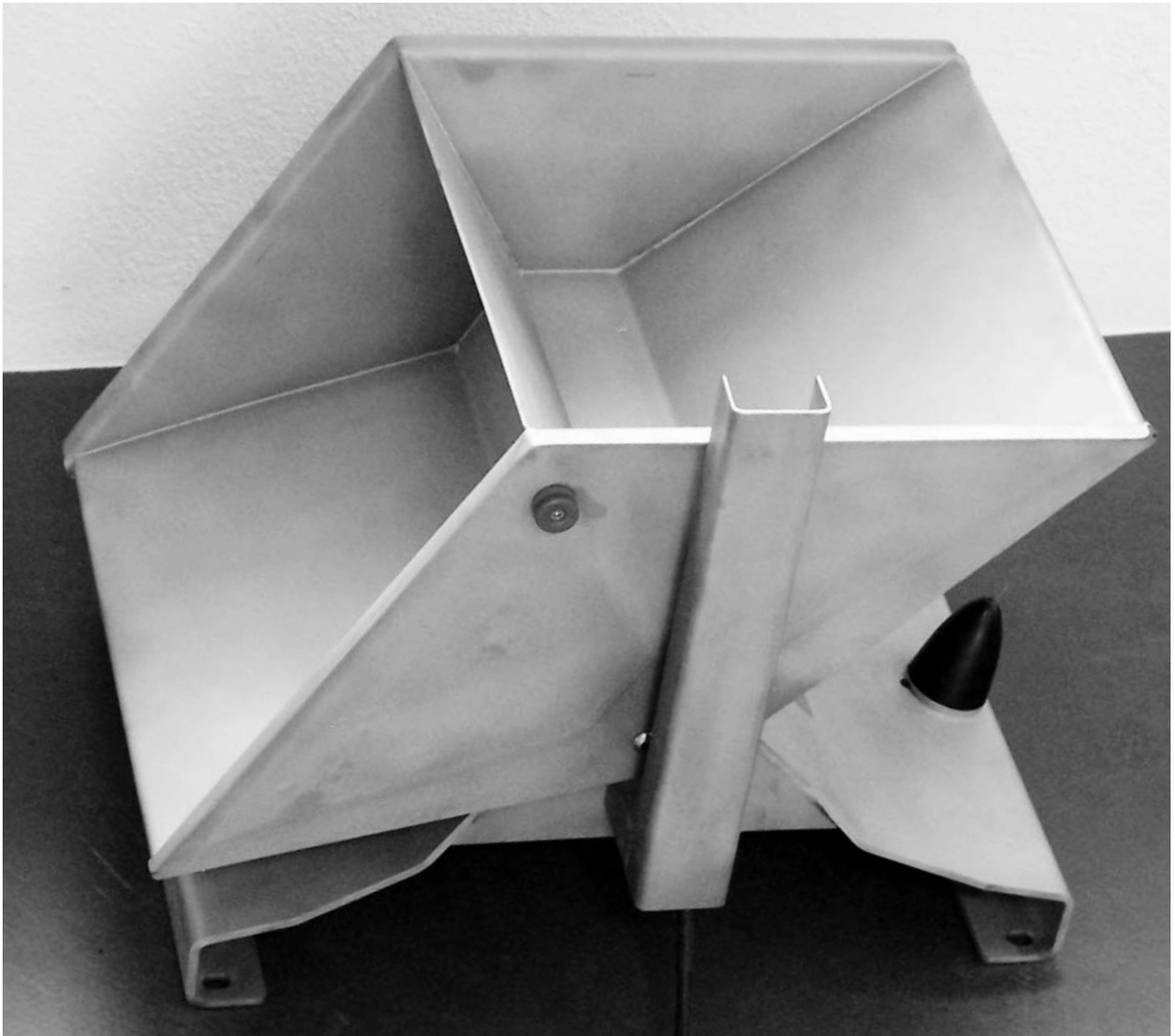
Fig. 2: Tipper Flow Measuring Device UFT-FluidTipper with a volume of 16 litre by double filling. The unit is fitted with a magnetic switch to detect each filling cycle.
