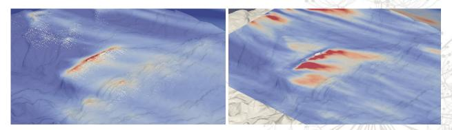
RANS model (left) shows clear underprediction of turbulence behind cliff. DES model better describes the physics of large scale recirculation.
