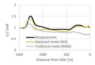
Model validation along a lidar line-of-sight clearly show shortfall of traditional RANS model in highly complex terrain. RANS model gives error in the order of 40%!.
