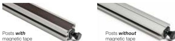
Posts **with** magnetic (mag) tape are used on the front of the counter and on the back outside corners. Posts **without** mag tape are used only on the back of the counter at intermediate sections, not on the corners.
