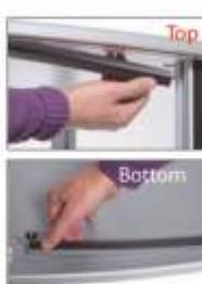
**9** Mount the magnetic strips provided along the top and bottom edges of each section where graphic panels will be added. Add corner trims on all outer corners.
