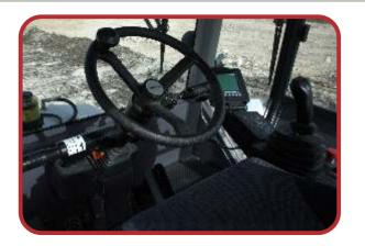
The operator station has an adjustable swivel seat with variable suspension for comfortable driving and excellent visibility in all directions.
