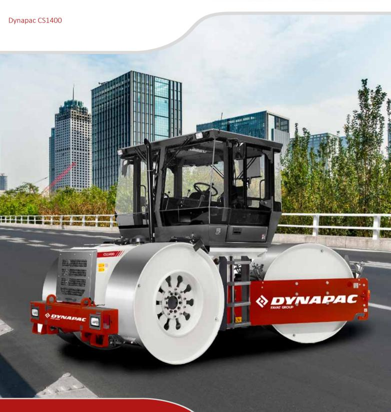
THE DYNAPAC CS1400 STATIC ROLLER is a modern, articulated three-drum roller with the same static linear load and drum diameter on all drums. The roller covers the asphalt mat with its full width. The CS1400 roller is used primarily to compact asphalt when the course has a typical thickness of up to 50 mm, depending on the stiffness of the asphalt compound and the prevailing weather conditions.
