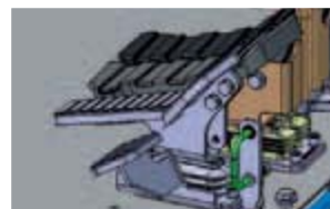
Straight travel pedal Allows more operator comfort when multi-tasking.
