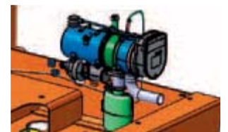
Engine coolant heater Improves start-up ability in extremely cold conditions by heating coolant and fuel.
