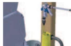
Air gun and compressor Clears dust inside cab and pump compartment. Cleans filter, radiator and oil cooler. Plugs available in cab, pump compartment and battery box.
