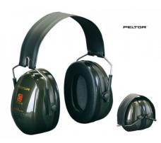
Type H 34/M 29/L 20, Sound Noise Reduction (SNR) 31 dB, weight 210 g.
