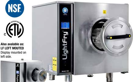
**Dimensions:** W27 x H29 x D25 inches Net weight: LF12C: 236 lbs **Electrical power:** LF12C: 3x220V+PE, 60Hz, 13kW Drainage conn: 1" inner diameter hose Fresh water conn: 3/4" Extraction options: Custom made standard ventilation hood or custom made
