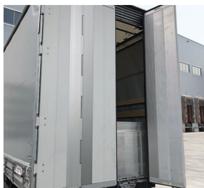
Sectioned portal on the bulkhead: the four-wing door enables the portal to be opened in the narrow space between the truck body and the trailer.
