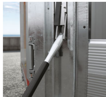
Manual lifting system integrated into the corner stanchions , flexible and reliable with built-in height adjustment.
