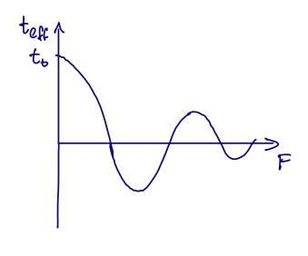
$|t_{eff}| \le t_0$  due to  $|J_o(x)| \le 1$
