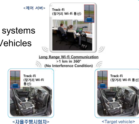
(Reference) Communications for Automated Vehicle assessment systems (Wi-Fi)
