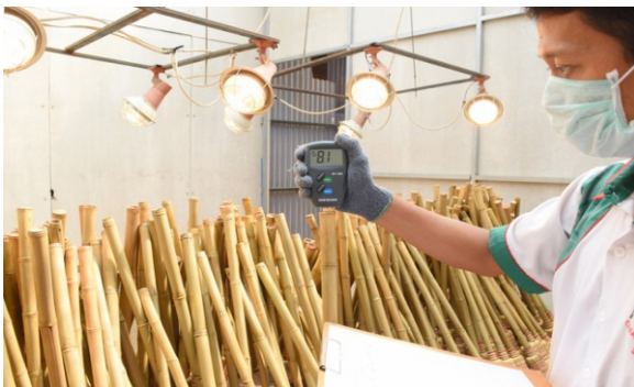
Water test to prevent mold growth
