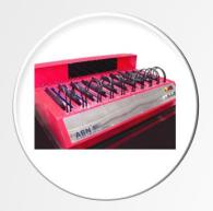
Bladder Leakage Test
