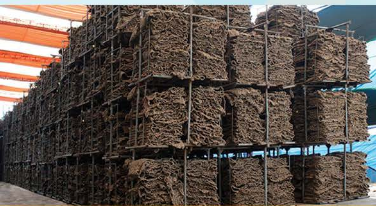
AGING BLANKET DRC USING METAL (WOOD-FREE) RACKING SYSTEM
