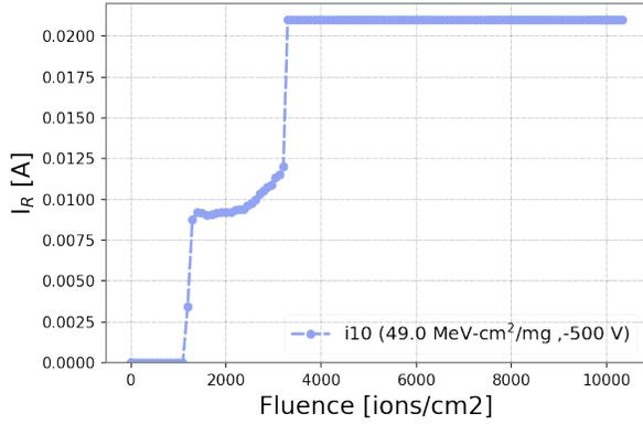
Fig. 13. Example of an SEB event for device *i10* for an ion LET of 49.0 MeV-cm<sup>2</sup>/mg at -450 V.
