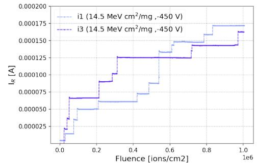
Fig. 7. Example showing discrete heavy ion induced steps in the leakage current during irradiation at -450 V for devices *i1* and *i3* at an ion LET of 14.5 MeV-cm<sup>2</sup>/mg
