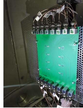
Fig. 6. Board 1 with 8 diodes mounted in the RADEF vacuum chamber.
