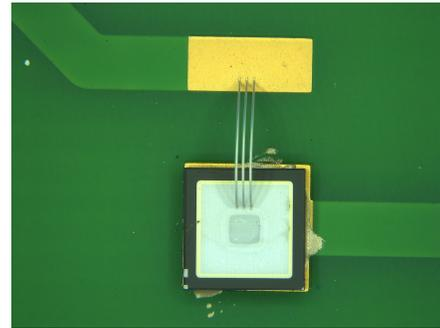
Fig. 4. The diodes were mounted directly on PCBs (cathode side down) using conductive silver epoxy. The anode side is connected to a nearby pad using three  $\varnothing 25 \mu\text{m}$  aluminum bonding wires, each expecting to support approximately 0.75 A. The bonding wires are assumed to be sufficiently thin to disregard beam shadowing effects.
