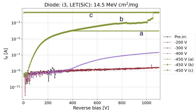
Fig. 12. Example showing reverse bias sweeps for device *i3* which was irradiated at an LET of  $14.5 \text{ MeV-cm}^2/\text{mg}$ . The values listed in the legend corresponds to the reverse bias voltages applied during the irradiation performed just before the IV-measurements. *Pre.irr.* refers to the IV-measurement performed before the device was irradiated. Three consecutive IV-measurements were performed after the  $-450 \text{ V}$  run.
