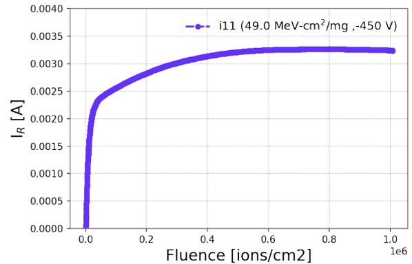
Fig. 14. Example of significant increase in leakage current for device *i11* for an ion LET of 49.0 MeV-cm<sup>2</sup>/mg at -450 V.
