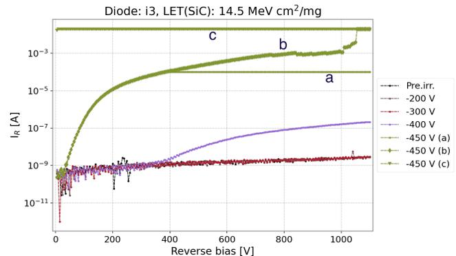
Fig. 12. Example showing reverse bias sweeps for device *i3* which was irradiated at an LET of  $14.5 \text{ MeV-cm}^2/\text{mg}$ . The values listed in the legend corresponds to the reverse bias voltages applied during the irradiation performed just before the IV-measurements. *Pre.irr.* refers to the IV-measurement performed before the device was irradiated. Three consecutive IV-measurements were performed after the  $-450 \text{ V}$  run.
