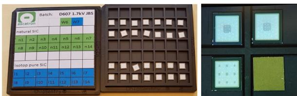
Fig. 3. Left: Box with bare die diodes, 14 natural SiC, and 14 mono-isotopic SiC. Right: Close up of 4 diodes, bottom right shows cathode/backside, the 3 others show anode/front side.
