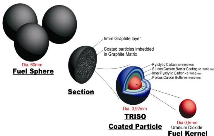
**Figure 2.** The balls containing nuclear fuel used in pebble bed reactors.
