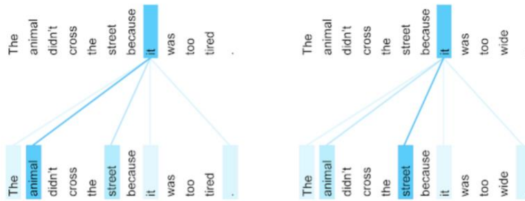
The encoder self-attention distribution for the word "it" from the 5th to the 6th layer of a Transformer trained on English to French translation (one of eight attention heads).
