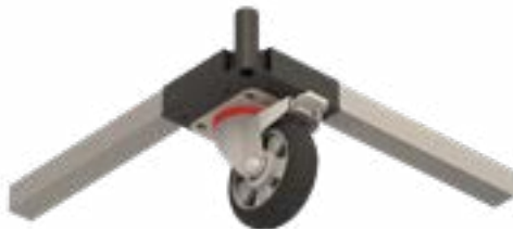
BQ160SB Swivel castor for Square Base with brake - load cap. 300 kg - diam. 160 mm
