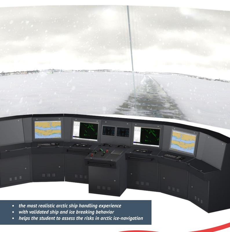
IS Full Mission Bridge Simulator for Arctic Operations is a comprehensive environment for training navigating in icy waters and fairways, designed to comply with IMO's arctic navigation training standard Polar Code. The validated ship and ice breaking behavior models are co-developed with Aker Arctic Technology Inc, the leading designer of arctic vessels.
