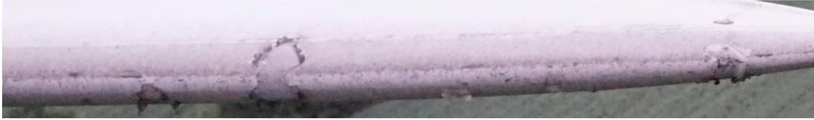
**Level 3 (LEP)** – “LEP is compromised over a large area and no longer providing protection to underlying layers”
