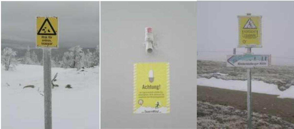
**Figure 8-2-2: Warning signs for falling ice. Photo credit Lars Tallhaug, Norway.**
