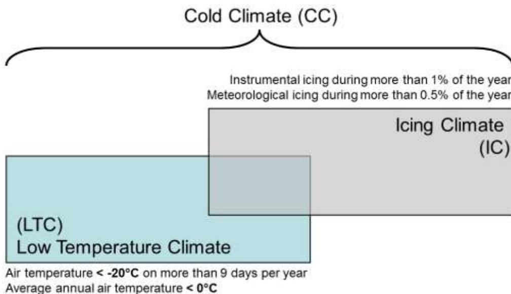
**Figure 2. Definition of Cold Climate, Low Temperature Climate and Icing Climate**
