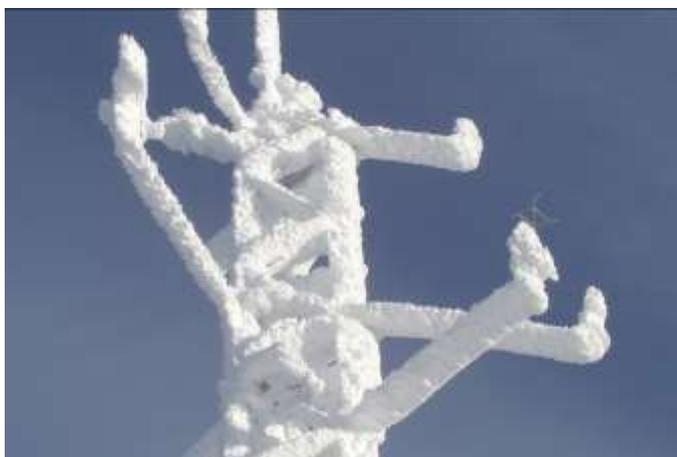
**Figure 4-2: The impact of ice build-up on mounting hardware and sensors must be considered to ensure the accuracy of wind speed and direction measurements. Photo credit: TMV2 Murdochville, TechnoCentre éolien.**
