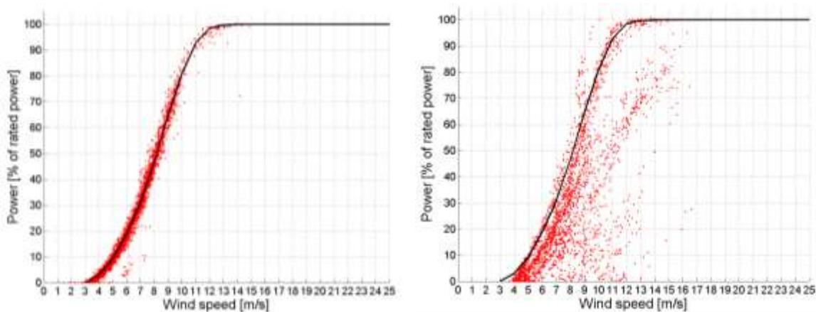
**Figure 7-3: Power (% of rated power) as a function of wind speed in two cases. On the left: A power curve registered in May 2010. On the right: An ice-impacted power curve registered in November 2009.**
