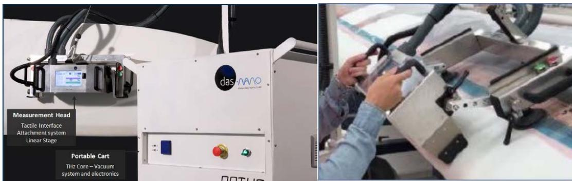
**Figure 51: (left) Notus system for non-destructive inspection of coating thickness and adhesion based on THz-TDS spectroscopy technology and (right) extended head position for leading edge inspection. On courtesy of das-Nano.**
