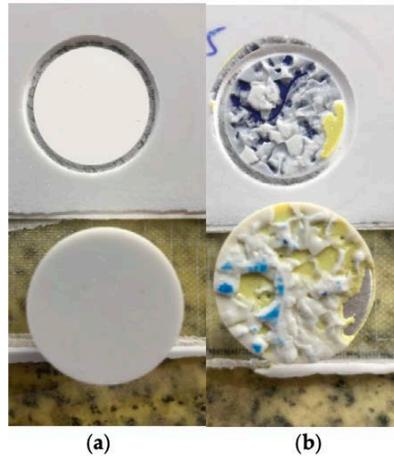
**Figure 32: Pull-off strength testing of specimen laminates used for LEP coating adhesion: (a) adhesive failure with no-primer intermediate layer application; (b) cohesive failure with primer application (the dolly adhesive effect can also be observed)**
