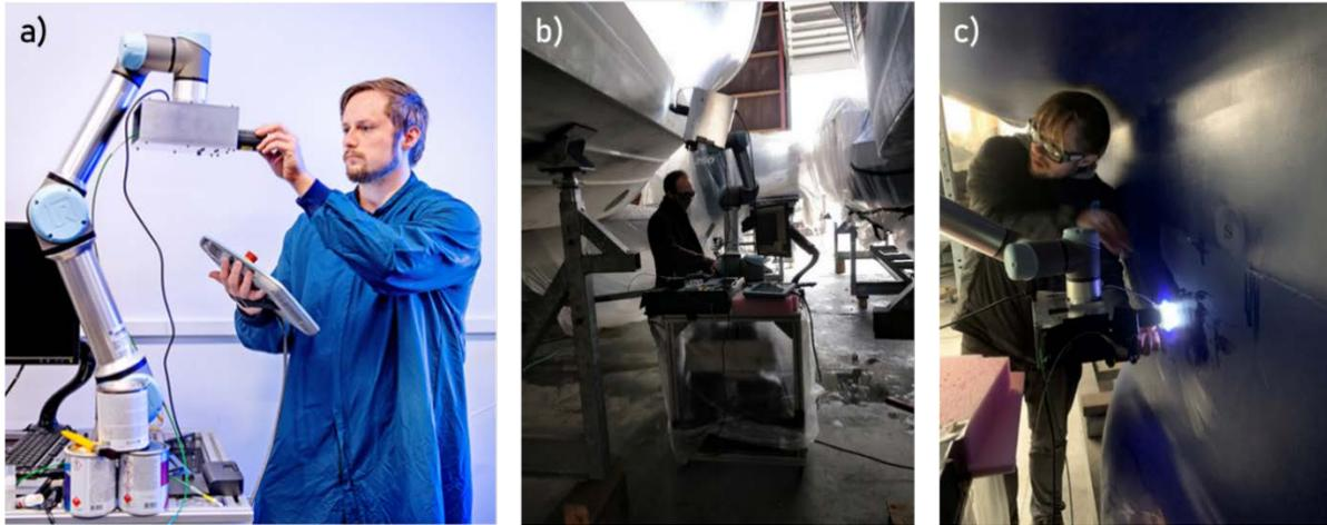
Figure 55. (a) Photograph by Bax Lindhart © 2021 showing the prototype being tested at DTU Fotonik. (b,c) OCT prototype in action scanning marine coatings directly on marine vessels at the Yacht Service wharf in Copenhagen, Denmark.
