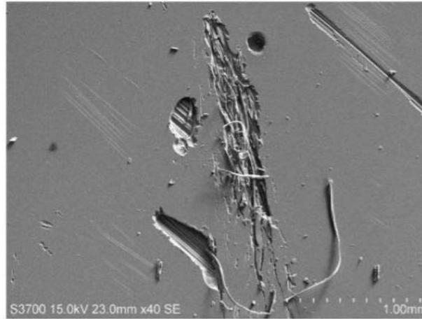
**Figure 46: SEM image showing fibre breakage observed after 50 impacts of 20mm hailstones at a velocity around 90m/s [Source: Macdonald2019]**
