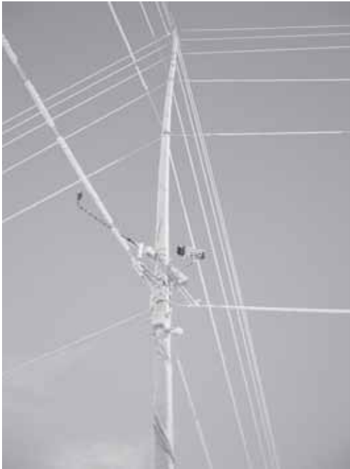
Figure 3 Wind measurements with video monitoring of icing in Norway. Photo: Kjeller Vindteknikk, Norway.
