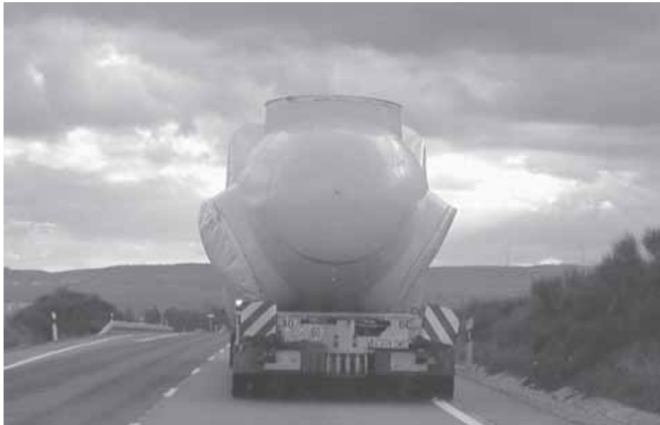
Figure 11 Transport of wind turbine nacelle.
