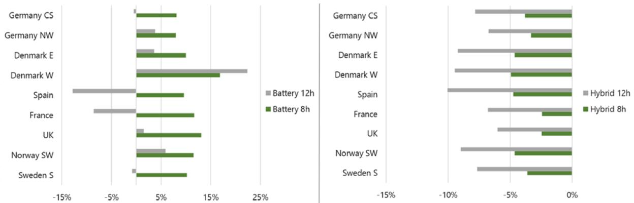
**Figure 19. Percentage difference in benefit-cost ratio<sup>4</sup> of the 8-h and 12-h configurations compared to the 4-h configuration for stand-alone batteries (left) and hybrids (right) in 2050**
