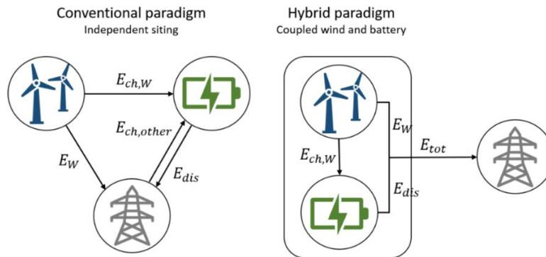
**Figure 3. Description of an independent sited system versus a hybrid system (E = electricity flow [generation/charge/discharge])**
