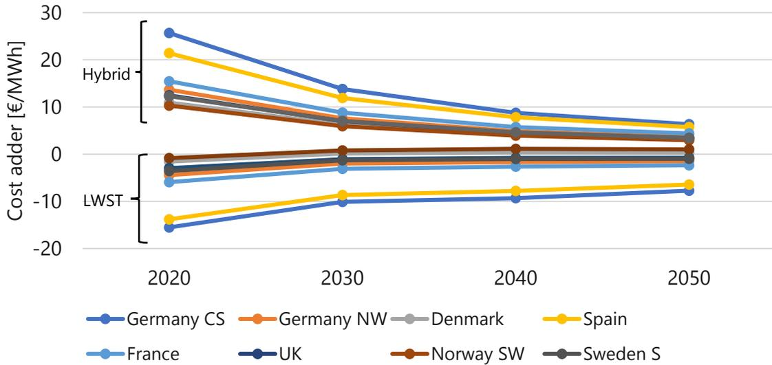
**Figure 26. Difference in LCOE (cost adder) for the hybrid and LWST, relative to the HWST**
