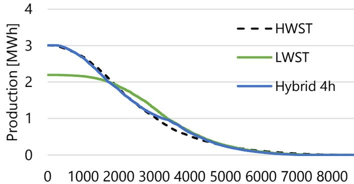
**Figure 24. Difference of the feed-in profile between a LWST and a 4-h hybrid (compared to the original HWST profile)**
