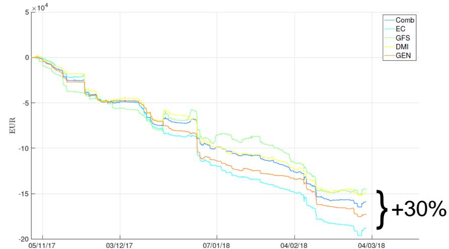
C. Hagberg, Vattenfall 2018: Verification of power prediction tools used for wind power forecasts - Cumulative imbalance costs HornsRev wind farm
