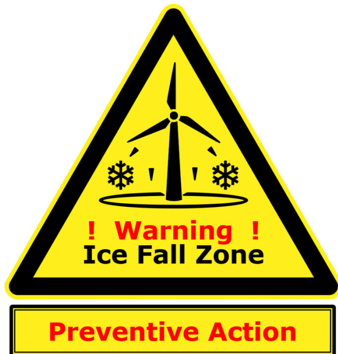
Figure 13: General warning sign for the risk of ice fall with an additional sign for a preventive action
