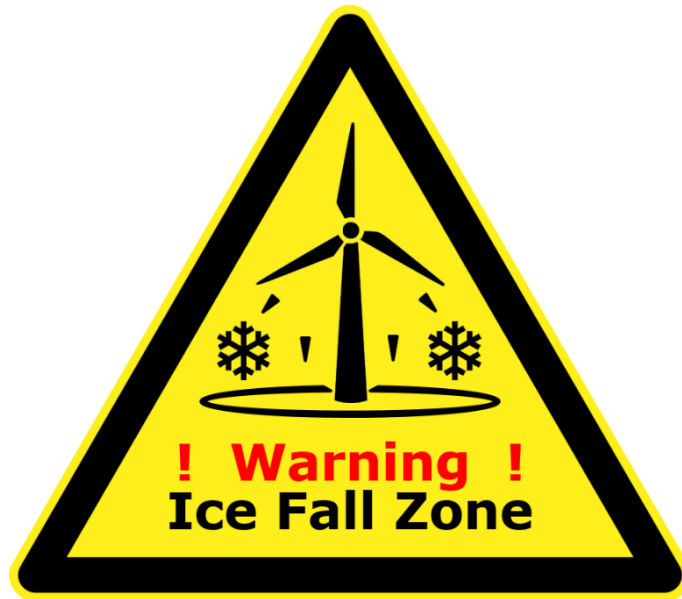
Figure 12: General warning sign for the risk of ice fall
