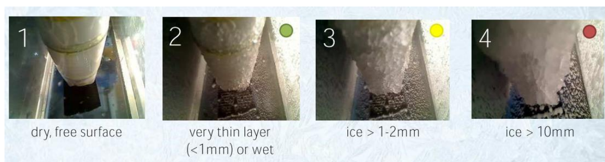
Figure 5: Lab validation of icing severity detection (Moser, 2017)
