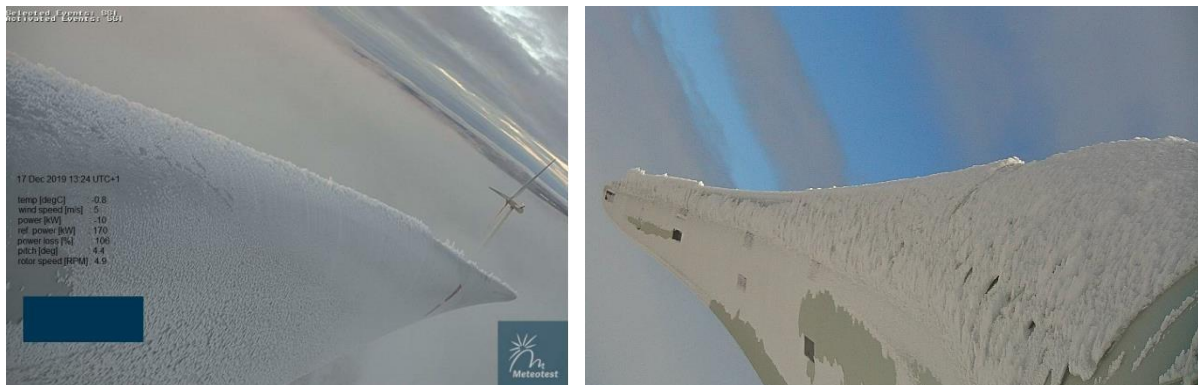
Figure 7: Validation of rotor icing detectors using images, by Meteotest in Sweden (left) and Nergica in Canada (right) (Froidevaux & Cattin, 2021) (Godreau, 2019)
