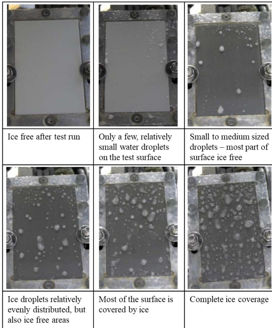
Figure 2-2. Reference pictures for ice formations on test surfaces (80 x 50 mm) after ice rain test at Fraunhofer IFAM with temperature -5 °C, wind speed 11.5 m / sec [4].
