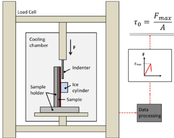
**Figure 2-7. Schematic illustration of the working principle of the vertical shear test [15].**
