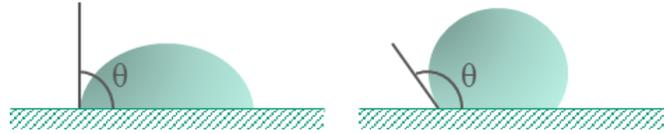
**Figure 4-3. Wetting of a surface by a droplet with contact angle  $\theta$  90° (left) and  $>90^\circ$  (right)**
