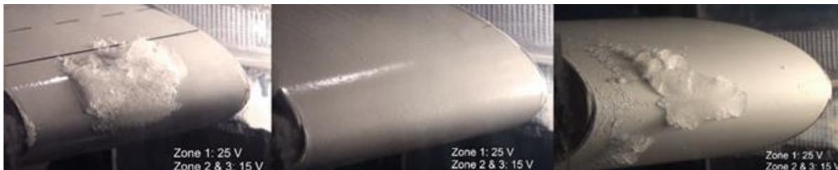
**Figure 2-11. Ice formation at leading edges of an aerodynamic profile with heating elements: unmodified PUR reference coating (left); elastomeric icephobic coating (center), superhydrophobic coating (right). (Source: Fraunhofer IFAM [4])**
