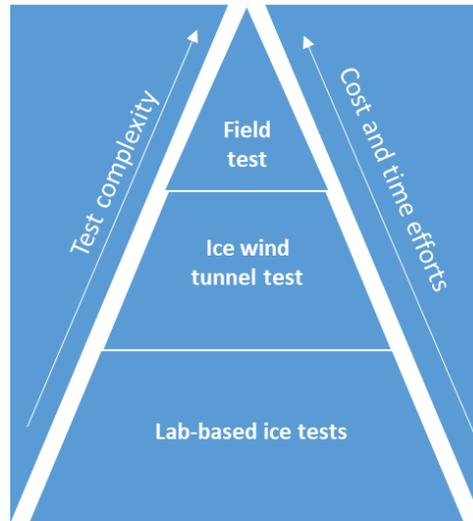
Figure 2-1. Scheme of ice-related testing during the development of icephobic coatings.
