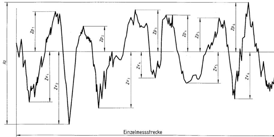
Figure 4-1. Example for a surface roughness profile [24].
