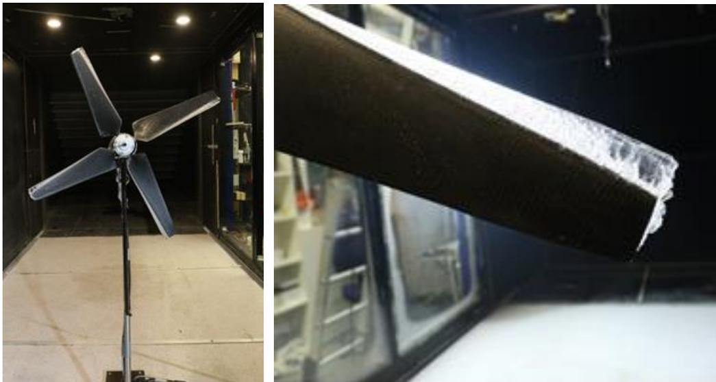
**Figure 2-10. Small wind turbine model in CWT with rotation speed control and a force balance at the base of the tower to measure the overall thrust of the rotor disc during icing and to compare the prediction from numerical simulation to experimental data [19].**
