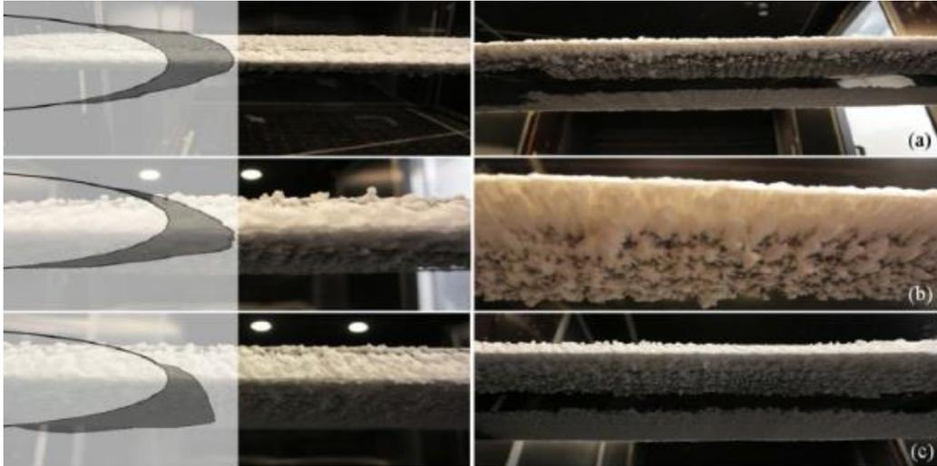
**Figure 2-9. Rime ice accretion at different pitch angles of the airfoil. (a) AoA - 0deg, (b) AoA - 5deg and (c) AoA - 10deg. Left – leading edge with contour trace of ice layer, right – leading edge close-up [18].**
