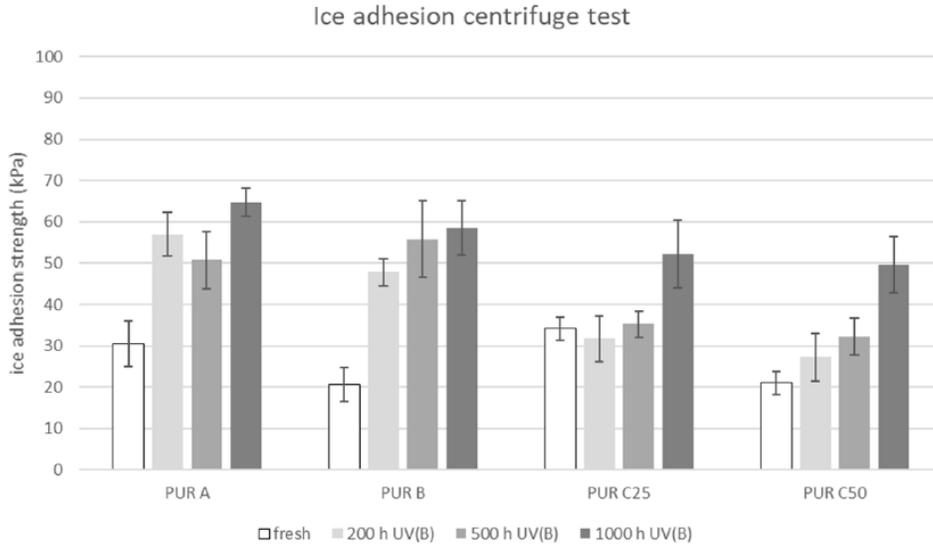
**Figure 3-1. Results of ice adhesion centrifuge test (kPa) for coatings prior to and after accelerated UV(B)-ageing, as indicated [14].**
