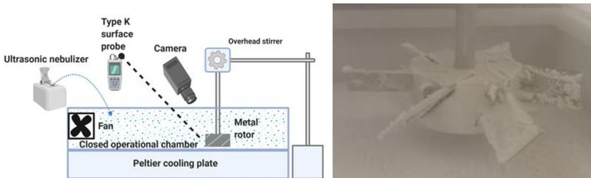
**Figure 2-4: A rotary dynamic icing lab test developed at University of Nottingham: schematic diagram (left) and ice accretion on the tested samples (right) [5].**
