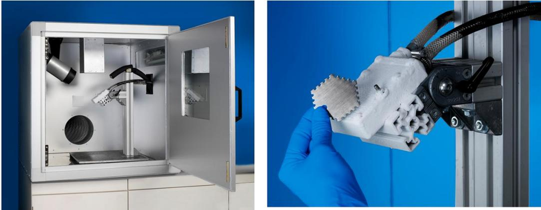
**Figure 2-3: Example for a test chamber for lab-based ice tests (left) and frost/rime ice accretion on a test surface (80 x 50 mm) at test surface temperature  $-2^\circ\text{C}$  and air temperature  $+1^\circ\text{C}$ . Wet film thickness gauge used for ice thickness measurement (source Fraunhofer IFAM) [4].**
