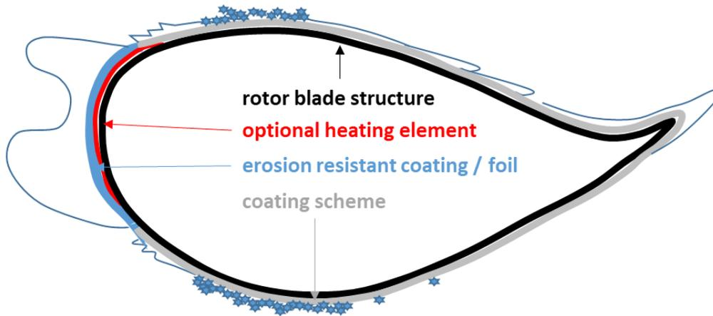
Figure 1-3. Scheme of a rotor blade with basic material scheme and ice formations to be expected. Aerodynamic profile taken from [22].
