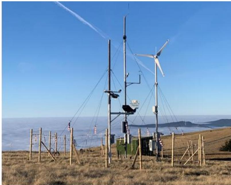
**Figure 2-12. Combined set-up for small-scale ice formation test (left) and dynamic test of coating/surface durability on the blades of a small wind turbine (right). Separate mast for overview camera and meteorological sensors (middle). (Source: Energiewerkstatt Verein)**
