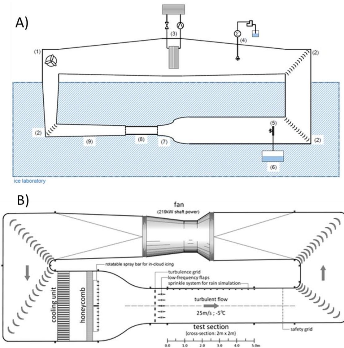
Figure 2-8. Examples for ice wind tunnel test facility: A – Fraunhofer IFAM with fan drive system (1), turning vanes (2), heat exchanger of refrigeration system (3), humidistat (4), water spray bar (5), water reservoir and pumps (6), test section entrance (7), test section (8), diffuser (9) and B – Overall layout of the cold climatic wind tunnel (CWT) airline at DTU. The wind tunnel is installed in vertical plane placing the fan above the 5m long test section.
