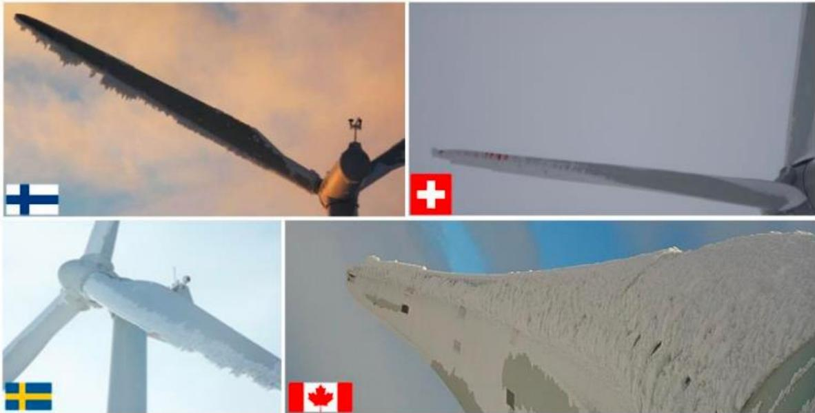
Figure 1-1. Icing on wind turbine blades in different parts of the world (source: Task 19)
