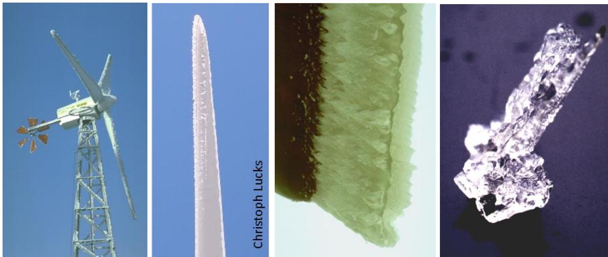
Figure 1-2. f.l.t.r.: Icing of wind turbines at stand still; Icing of wind turbines during operation; Rime ice at the leading edge; Glaze ice from rotor blade icing. All pictures from [3].
