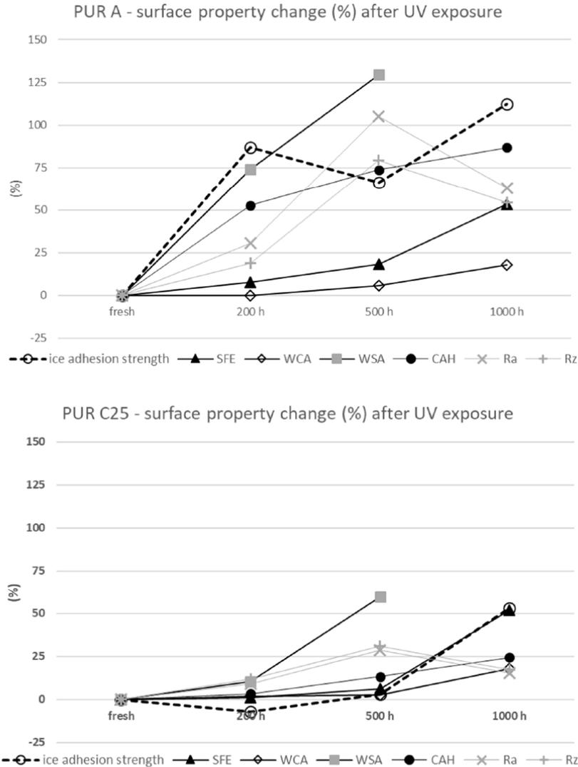
Figure 4-5. Change in surface properties and ice adhesion strength (%) due to UV(B)-ageing for exemplary coatings [14].
