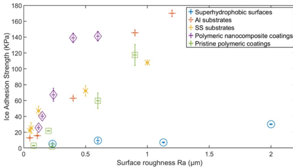
Figure 4-2 Ice adhesion strength on variable surface roughness  $R_a$  for different material types [25].
