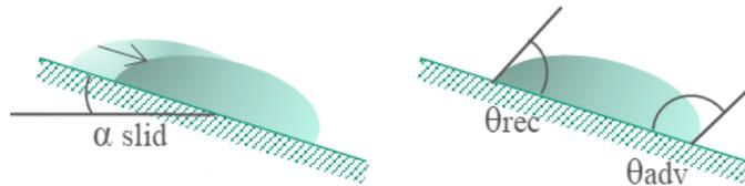
**Figure 4-4. Water droplet sliding angle  $\alpha_{\text{slid}}$  (left); receding  $\theta_{\text{rec}}$  and advancing  $\theta_{\text{adv}}$  contact angle of a droplet (right).**
