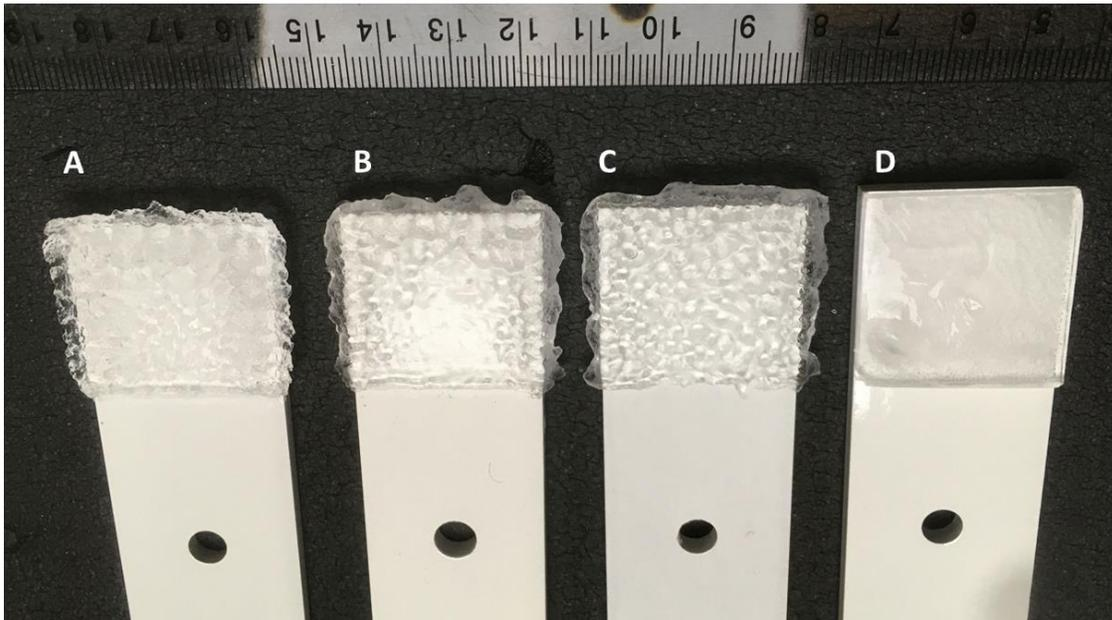
**Figure 2-5. Ice types generated in ice wind tunnel at velocities of 95 m/s (A), 60 m/s (B), 40 m/s (C) and generated by filling liquid water in a mould to freeze at the test surface (D), respectively; all ice formations at temperature of -8°C (source: Fraunhofer IFAM).**
