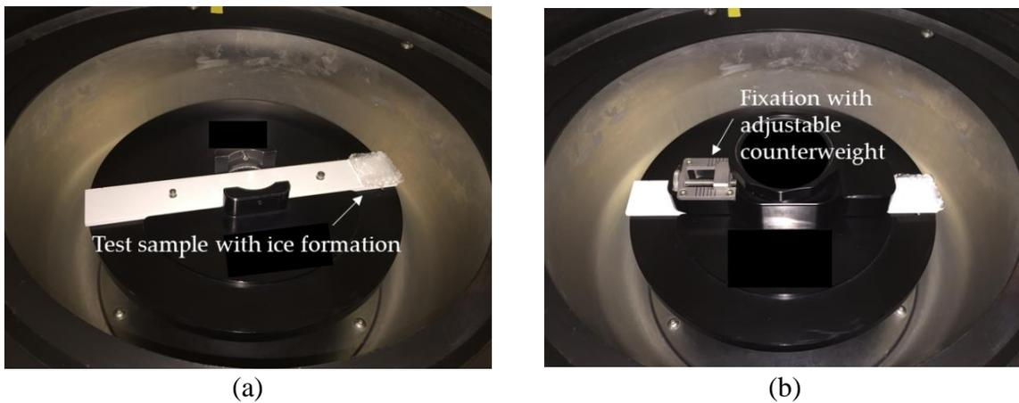
**Figure 2-6. View inside the centrifuge test device with: (a) test sample with ice formation placed in the centrifuge; (b) test sample after fixation. (source: Fraunhofer IFAM)**
