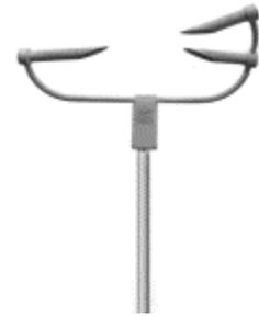
The OTT Parsivel-2 and Thies Laser Precipitation Monitor (LPM) disdrometers work on a similar measurement principle and measure hydrometeors as they fall through, and thus break, a series of adjacent horizontal beams. The Thies disdrometer uses a wavelength of 785 nm, while the OTT Parsivel<sup>2</sup> uses radiation with a wavelength of 650 nm. The
