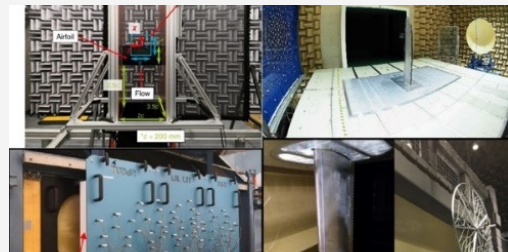
Serrated airfoils are measured in different wind tunnels (DTU/DLR-DNW/TU Delft) - Results are being compared.
