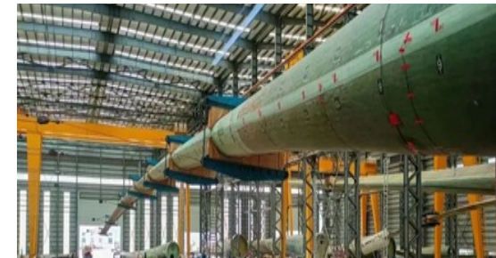
103m long blade passed the static test
