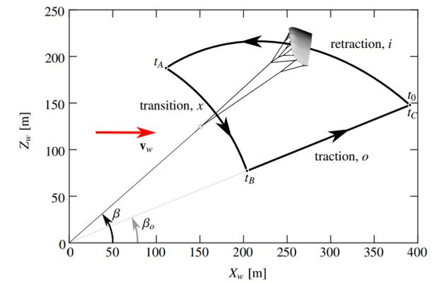
Source: Van der Vlugt et al. – Quasi-Steady Model of a Pumping Kite Power System
