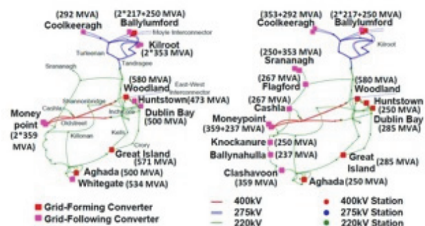
Fig. 11. Ireland power system simulations for MIGRATE project: an "urban" distribution for the grid-forming and grid-following converters on the left and a "remote" distribution on the right [33].
