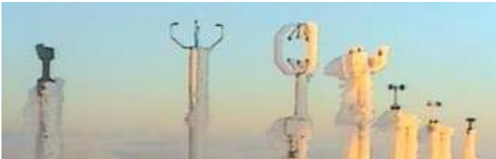
Figure 5. Testing different wind anemometers in severe icing climate (source: [42])
