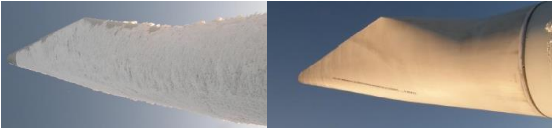
Figure 10. Blade without (left) and with (right) ice protection system (source: VTT)
