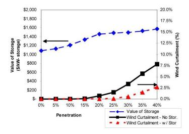
**Figure 2.** Value of storage will increase when share of wind increases. At higher shares of wind power, storage capacity will also reduce curtailments needed for wind power in situations where wind is high and demand is low. (Source: LBNL, US).
