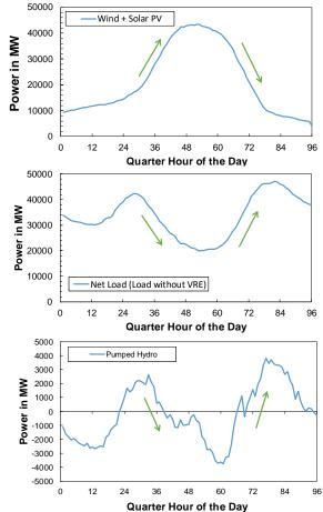
**Figure 1.** Pumped hydro power plants already see a change in their daily pattern for pumping (negative) and generating (positive) in Germany (8 Aug 2019). VRE=Variable Renewable Energy. (Source: FfE, from ENTSO-E data).
