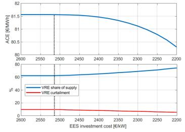
**Figure 3.** As the cost of storage decreases, it becomes cost effective to install storages to absorb wind and solar curtailment, and thus increase the cost effective share of wind and solar in the system. ACE=Average Cost of Electricity for the power system, EES=Electric Energy Storage, VRE=Variable Renewable Energy. (Source: Korpås & Botterud 2020).
