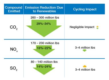
**Figure 4.** The increase in fuel consuming plant emissions from cycling to accommodate variable renewables is very low compared to the overall reduction in  $CO_2$ ,  $NO_x$ , and  $SO_2$  due to adding renewables. (Source: WWSIS2, 2013) (1 million lbs = .45 million kg).
