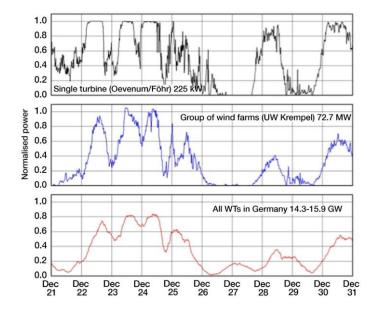
*Figure 1.* Short-term power output variations of a single turbine (top) are smoothed when aggregated with a group of wind power plants (middle). Aggregating the output from all turbines across Germany (bottom) smoothes the variations even more. As seen in the middle plot, the power generation from a small area can sometimes exceed the installed capacity. (Source: Task 25 summary report, 2009)).
