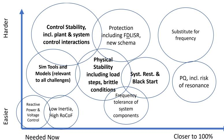
FDLISR fault detection, location, isolation and recover; RoCoF Rate of Change of Frequency PQ Power Quality
