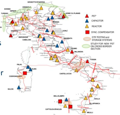
Example of grid investments to active and reactive power management in Italy (DTR = dynamic transmission rating). (Source: Terna)
