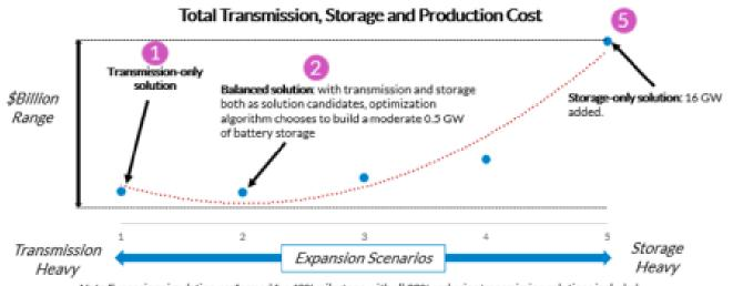
comparison of transmission-only solutions, storage-only solutions, and combined transmission/storage solutions for 40% wind and solar in Eastern Interconnection of the US (source: MISO RIIA)
