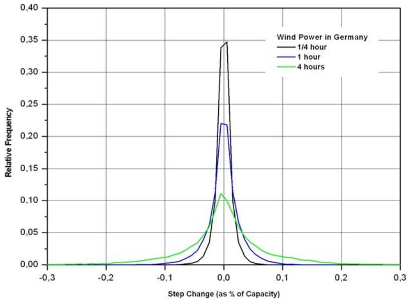
Fig 4. Frequency of relative power changes in  $\frac{1}{4}$ , 1 and 4 hour intervals, Germany, 01/01–31/12/2004 (ISET, 2005). A positive value reflects an increase in power and a negative value a decrease.
