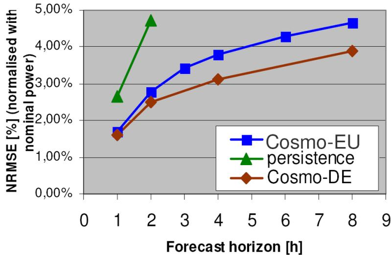
Fig 10. The latest prediction models can improve considerably also the short term production forecasts of wind power. Normalised RMSE error for the wind power production forecast for Germany using two (Cosmo-DE and Cosmo-EU) data as input. Additionally the persistence is shown for the first two hours (Wessel et al., 2008).
