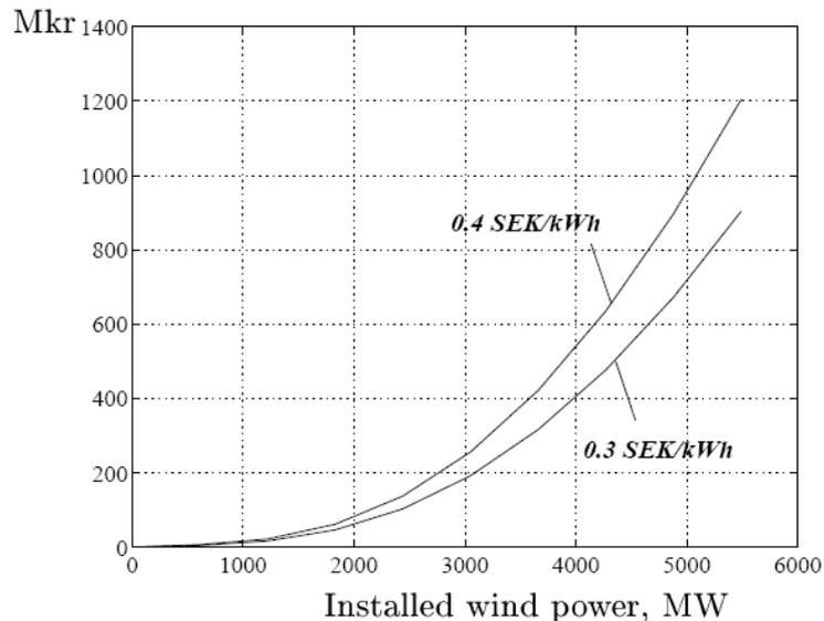
Fig 35. The cost for the spillage as a function of installed amount of wind power for two price levels of the spillage.
