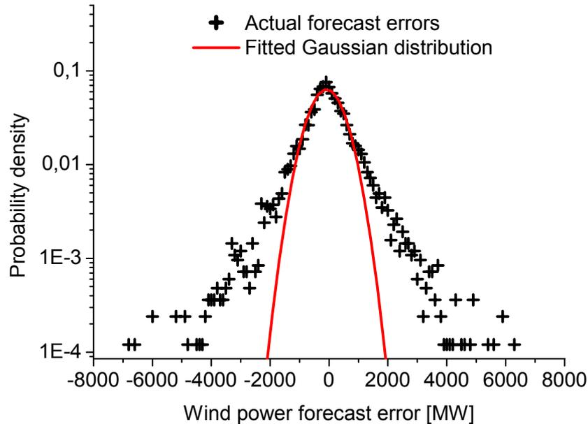
Fig 11. Probability density distribution of errors for the day-ahead wind power forecast for Germany; also shown is a fitted Gaussian distribution. (Source: Lange et al., 2006.)
