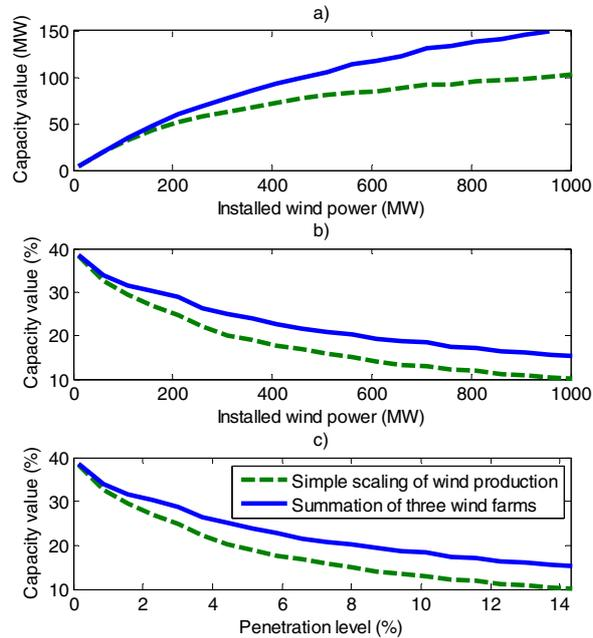
Fig 45. Capacity value of wind power with and without geographical smoothing effect. a) Capacity value in MW. b) Capacity value in percentage of installed wind power. c) Capacity value as a function of wind penetration level.
