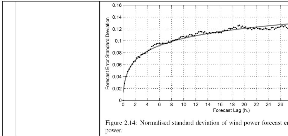
Figure 2.14: Normalised standard deviation of wind power forecast error.
