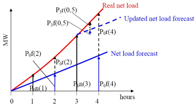
Fig 18. Need of “Flexibility” is the need for some units to follow the “net load variability”, marked  $P_{kn}(t)$ . This can be partly done by units scheduled beforehand, to follow the “net load forecast”, marked  $P_{kf}(t)$ , while “reserves” is the need for some units to follow the “net load forecast errors”, marked  $P_{kr}(t)$ .
