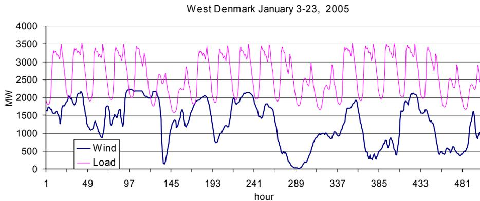
Fig 1. Wind power production (2 400 MW wind power) and load in Western Denmark. The storm event of 8<sup>th</sup> January can be seen in hours 128–139. (Data source: <http://www.energinet.dk>.)
