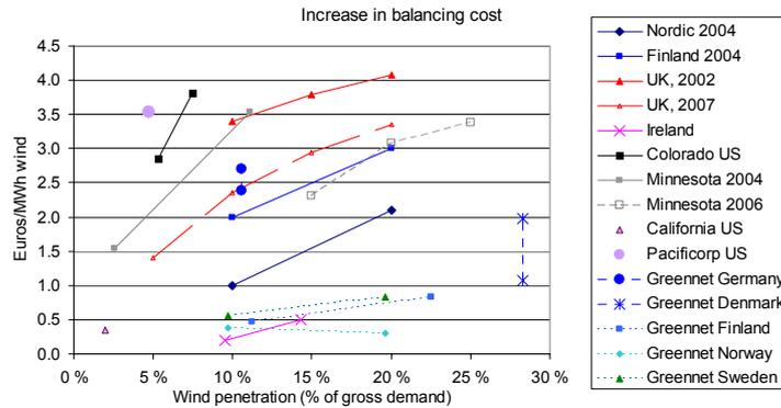
Fig 57. Results from estimates for the increase in balancing and operating costs due to wind power. The currency conversion used here is 1 € = 0.7 £ and 1 € = 1.3 US\$. For UK, 2007 study the average cost is presented here, the range in the last point for 20 % penetration level is from 2.6 to 4.7 €/MWh.
