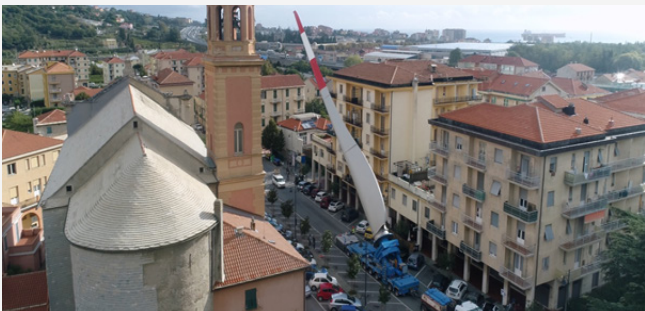
Blade Lifter transport system through a small village to the site of installation of Rocche Bianche wind plant (credit: FERA Srl).
