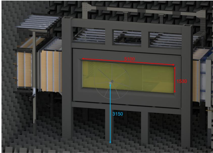
Figure 8: Rendering of the acoustic setup.
