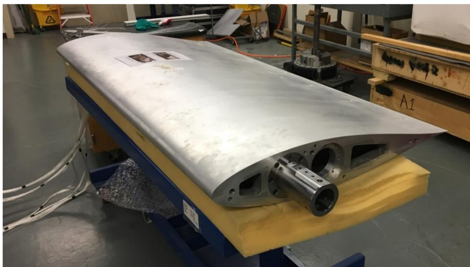
Figure 1: The large NACA63-018 aerofoil model.
