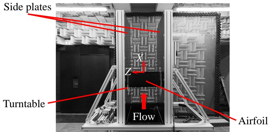
Figure 9: The A tunnel.
