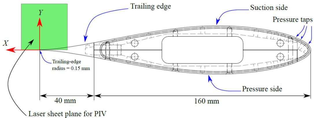
Figure 3: The small NACA63-018 aerofoil model.
