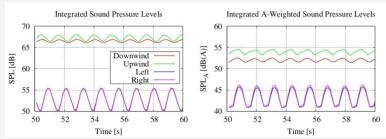
Figure 3. Time-series of integrated SPL showing amplitude modulation due to rotation of the blades and directivity effects illustrated by four listeners' locations relative to the wind turbine (Left: sound pressure levels, Right: A-weighted sound pressure levels)
