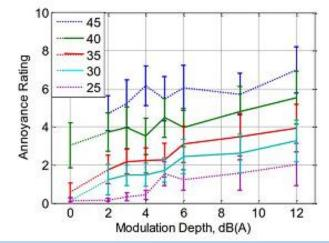
Figure 8. Relationship between modulation depth and annoyance rating with overall average level ( $L_{Aeq}$ ) as a parameter. From von Hünerbein et. al. Reference 11 WP 2(B)
