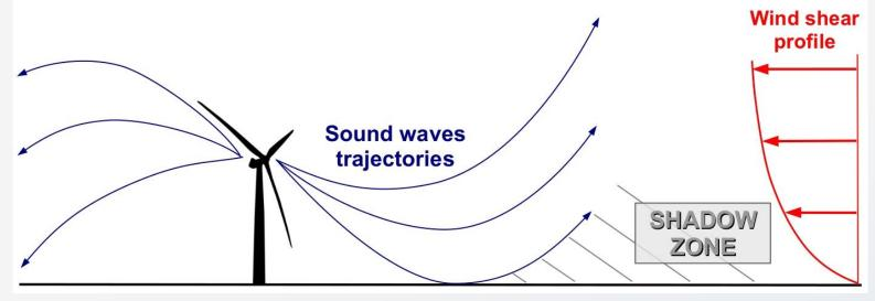
Figure 6. Shadow zone for the noise produced by a wind turbine
