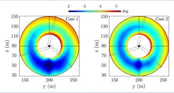
Figure 5. Time-averaged angle of attack across the rotor plane with the same hub height wind speed for two wind shear examples: high shear left and low shear right. See Reference 6.
