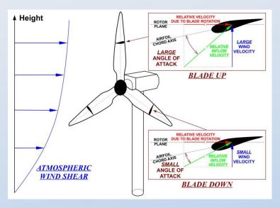
Figure 4. Sketch illustrating the varying angle of attack of the relative velocity impinging on a blade section as it rotates within the atmospheric wind shear
