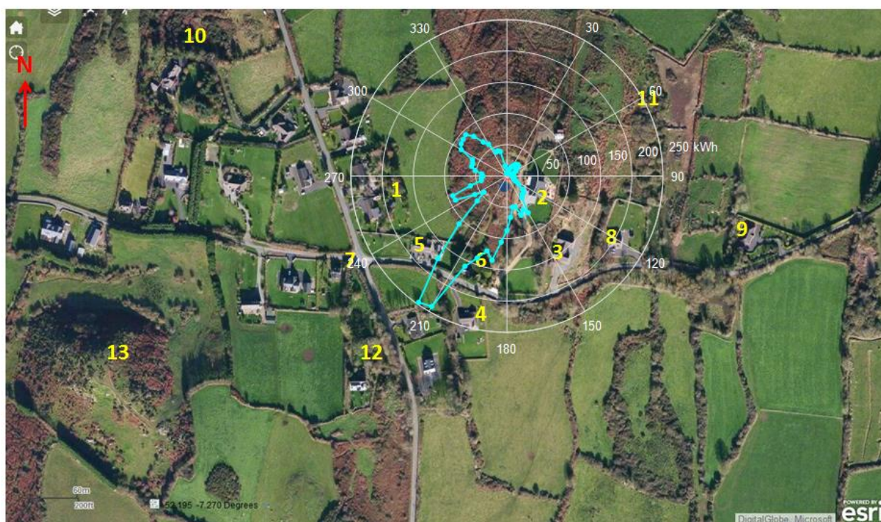
Figure B.8. Electrical energy rose overlaid on Site A plan view with numbered obstacles
