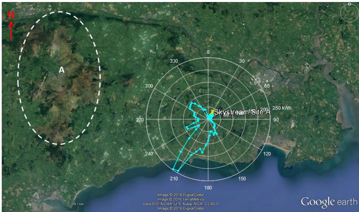
Figure B.9. Electrical energy rose overlaid on regional plan and labeled topographical features
