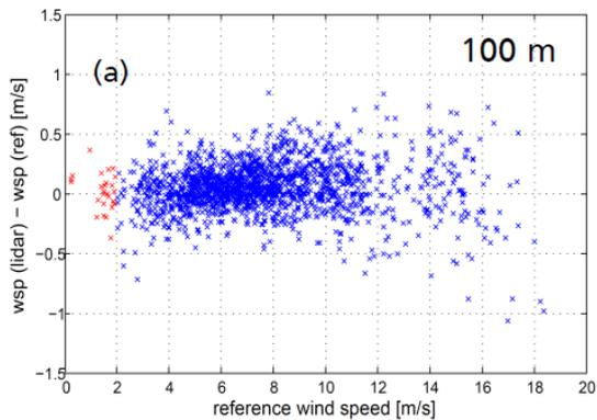
(d) Example of wind speed error sensitivity to wind speed (Reference 9).
