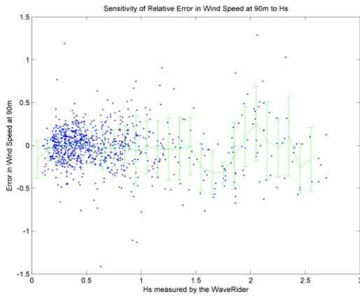
(a) Example of wind speed error sensitivity to significant wave height (Reference 8).
