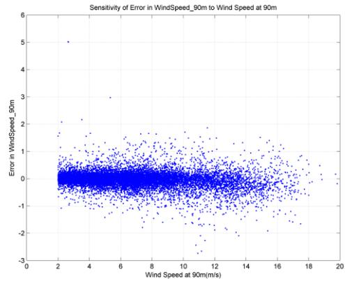
(b) Example of wind speed error sensitivity to wind speed (Reference 14).
