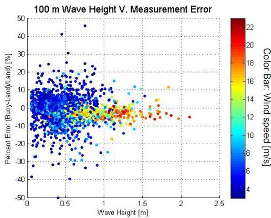
(c) Example of wind speed error sensitivity to wave height (Reference 6).
